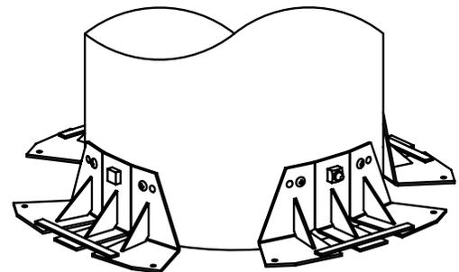
One or two pairs of pole bearing plates can be used. Plate only Catalog No. C1100954\*
