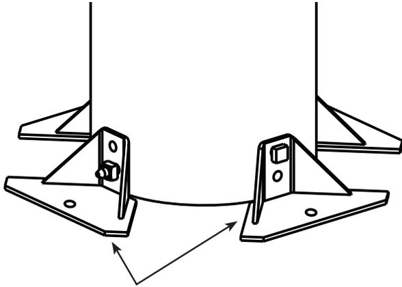
One or two pairs of pole bearing plates can be used. Note how each pair mounts with one bolt through upper or lower locating hole.
