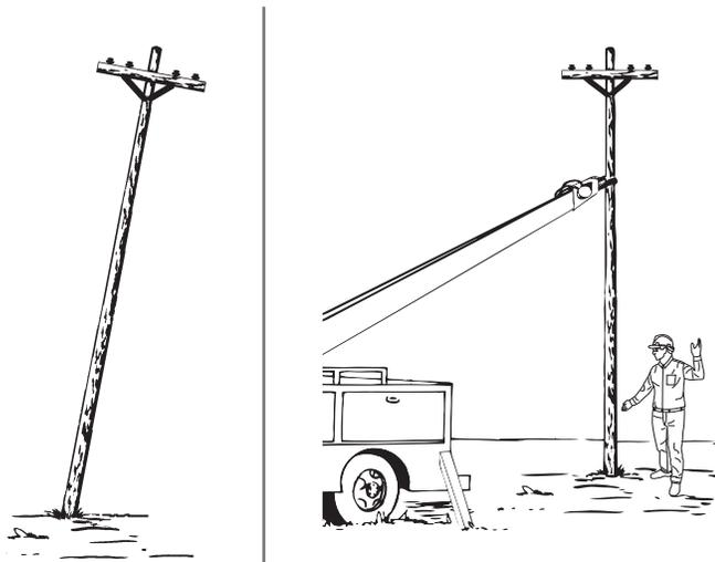
Chance Pole Key anchor is quickly installed next to a pole butt to help hold it in place against light overturning loads due to service drops, prevailing winds or small changes in line direction (See illustrations).
