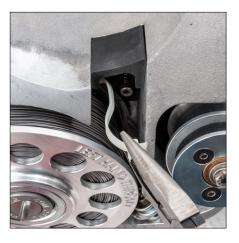
8. Remove the remaining cable tie.
