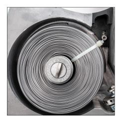
**5.** Cut and remove the 3 wire ties that were not rotated.
