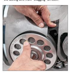
**9.** The reel brake can be depressed into cutout on rear flange to hold the reel stationary as you tighten the reel cover.
