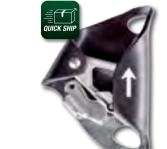
3/8" - 1/2" (9 - 13 mm) rope diameter. Compact and lightweight. Cam is spring-loaded and fitted with a catch mechanism. Easy for onehanded operation. Increased grip at low load, even on wet, greasy, oily ropes. Cam made from stainless steel for greater durability.
