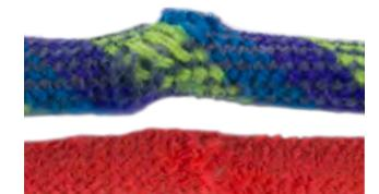
Pictures above showcase damaged rope cores and frayed/abraded sheath
