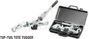
Solid steel construction, heavy-duty, dual ratchet drive design. 7.5' reach, 3,000 lbs pull capacity. 1,500 lbs lift capacity. 3/16" cable diameter. 6' double line lift height. 12' cable length. Folds into compact carrying case, folding handle.
